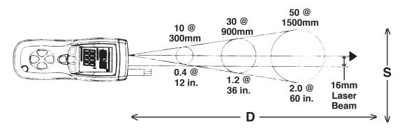
As the distance (D) from the object increases, the spot size (S) of the area measured by the unit becomes larger. The relationship between distance and spot size is listed on the diagram above. The focal point is 914mm (36"). The spot sizes indicate 90% encircled energy.
